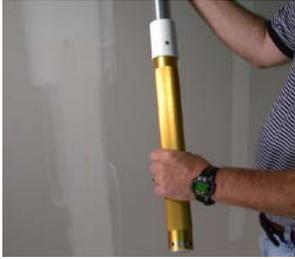
Control tube cap needs to be lubricated
