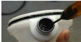
Clean filler valve and gently remove any debris that could be keeping the valve open. Be careful not to damage the filler spring.
