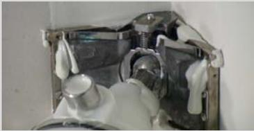
Joint compound is too thin and flow of joint compound is too fast.
