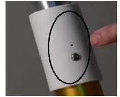
Rod wiper is dry and needs lubrication (top of tool near needle plug)
